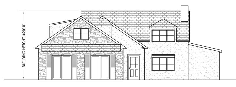
2 \ FRONT ELEVATION Z1 | SCALE : 1/4" = 1' - 0"
